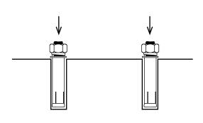
Step 3. Remove nuts and washers from the expansion anchors, and align the mounting holes with anchors to install the metal bollard body to the desired location.
