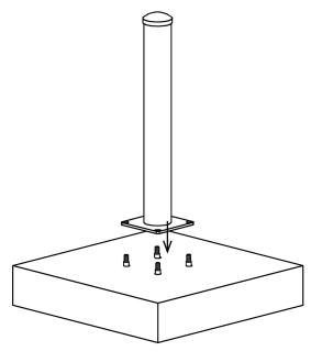
Step 4. Secure the bollard by tightening nuts with flat washer and lock washer to the installed anchors.
